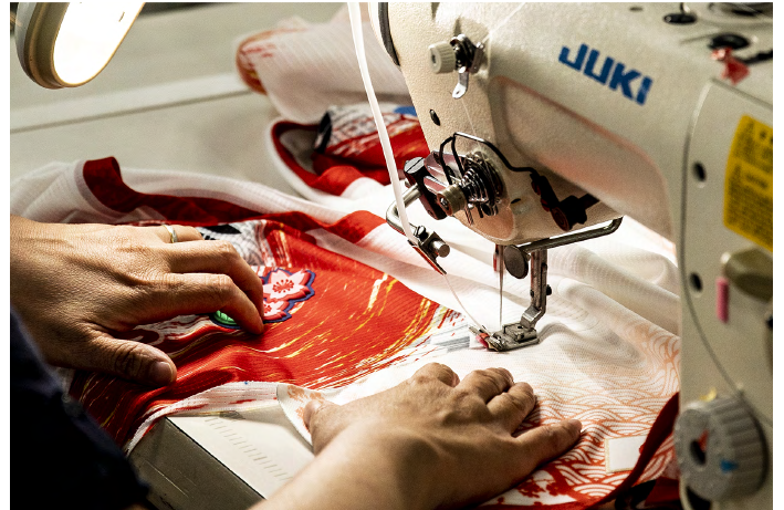
SMART SEAM® is an original GOLDWIN technology. Creating flat seams to reduce seams' stress on the skin
